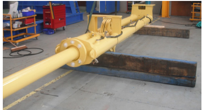
Heave Compensated System Rebuild
